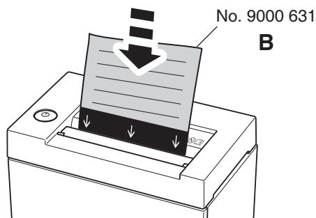
If the sheet capacity reduces or after the shred bin is emptied oil the shredding mechanism! (see picture)
