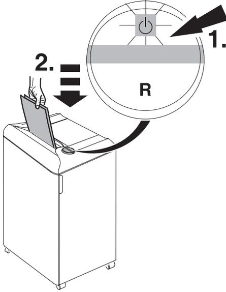
Reset by pressing the rocker switch ⏻.
