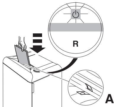
Feed the paper into the centre of the feed opening? (photo cell) (A)
