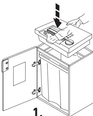
Open the door and put the machine onto the cabinet so that the control panel is facing the door. Beware of fingers.
