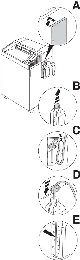
Installing the oiler:
