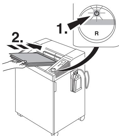
Is the rocker switch pressed? The green light rocker switch is ON? (1.). Insert paper (2.).
