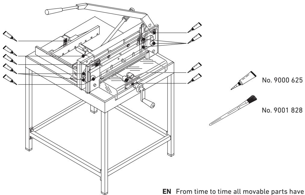
**EN** From time to time all movable parts have to be lubricated (use special grease for cutting machines). All paper and dust should be removed, as well as any grease.
