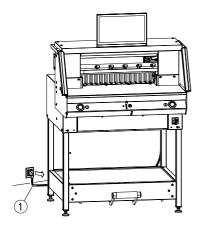
Protect the power cable 1 from heat, oil and sharp edges!
