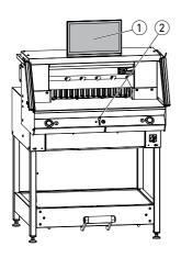
The dimension is set manually by way of the operating control for the electrical back gauge adjustment 2 or by way of programming the cutting size at the multi-touch display 1.
