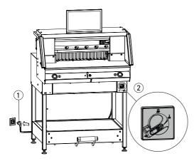
Plug in power cable ① at the power socket. Ensure free access to mains. Main switch ② at Position "I". The reference point for the back gauge is automatically moved to. The machine is operational.
