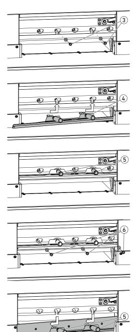
• Unscrew 2 blade screws (3) (with open slots).
