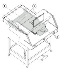
Paper installation at the back gauge 1 and side stop to the left and right 2. Use the provided paper knock-up block 3 for adjusting paper stacks.
