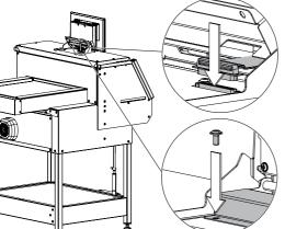
• Carefully insert display flat cable into the appropriate machine socket.
