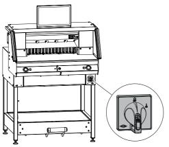
Shut down if not in use for a long period. (Main switch to "**0**").
