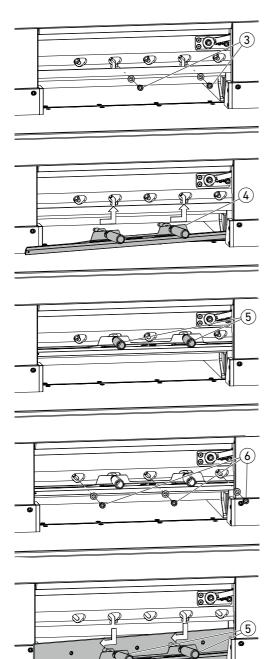
• Unscrew 2 blade screws (3) (with open slots).
