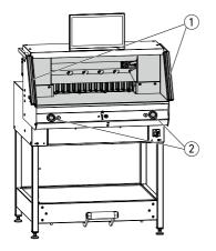
The dangerous cutting movement is protected by a safety light beam curtain (1) and a twohand cutting (2) activation!
