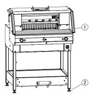
The adjustable feet (2) are used to level the machine and effect height adjustments:
