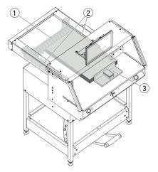
The dimension is set manually by way of the operating control for the electrical back gauge adjustment (2) or by way of programming the cutting size at the multi-touch display (1).
