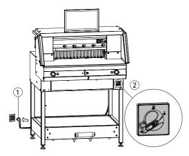
Plug in power cable ① at the power socket. Main switch ② at Position "I". The reference point for the back gauge is automatically moved to. The machine is operational.
