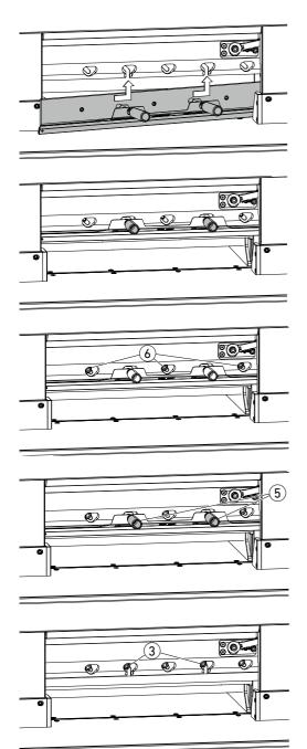
• Through the open slots, position blade with blade changing device at the top well over on the left and use the grips (5) for tightening.
