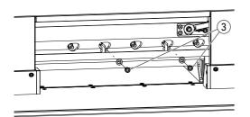
• Unscrew 2 blade screws (3) (with open slots).
