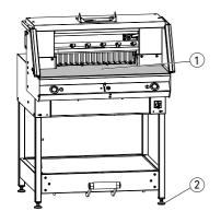
The adjustable feet (2) are used to level the machine and effect height adjustments:
