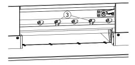
• Loosely screw in the remaining 2 screws (3). Remove all tools from the working area.
