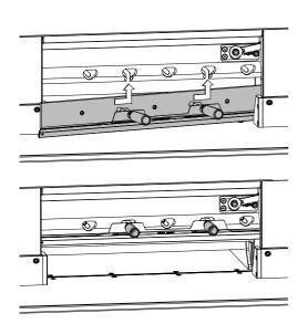
• Through the open slots, position blade with blade changing device at the top well over on the left and use the grips (5) for tightening.
