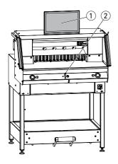
The dimension is set manually by way of the operating control for the electrical back gauge adjustment ② or by way of programming the cutting size at the multi-touch display ①.
