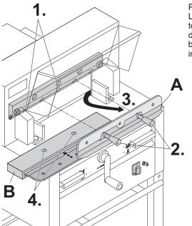
Remove 2 blade screws (1.). Loosen the grips (2.) of the blade changing tool (A) lightly and allow the blade to be taken downwards out of the machine (3.). Place the blade into the blade carrier (B) and screw it into place (4).
