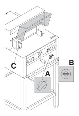
Position the main switch 4 to "I" (**A**). Insert the key 6 for the control system and move it to the right (**B**). Open the safety guard 6 (**C**). The machine is now ready for use.
