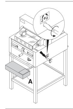
Turn the blade depth adjustment screw to the left until it stops. (Screwdriver found in tool set) (A).
