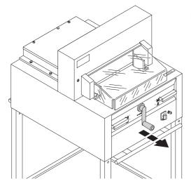
Pull out the handle to avoid the measurement being wrongly adjusted.
