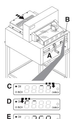
The measurement is set with the backgauge crank.(A) The symbol – rotary direction – ¬¬ moves to the right on the display (B) (see picture C). The rotary direction of the backgauge crank (A) is indicated on the right. Keep turning the backgauge crank to the right until a measurement appears (see picture E). The reference position is reached. The cutting size can now be set with the
