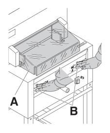
The dangerous cutting movement is safeguarded by a movable guard (**A**) and a safety two-handed control system! (**B**)
