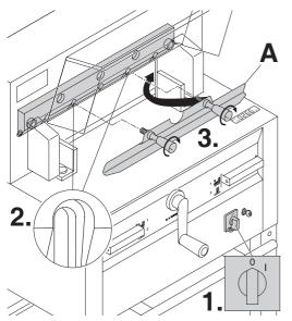
Position the main switch to "0" (1.) Remove the 2 blade screws on the elongated holes (2.). Then put the blade changing tool (A) into place and fasten it to the blade (3.).
