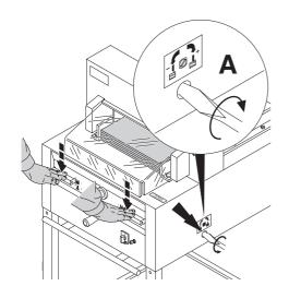
Paper cutting test. If the last sheet or several sheets are not completely cut, gradually turn the knob for blade depth adjustment (A) ¼ turn to the right until the paper is cut along the entire length. Do not set too low as blade will become blunt sooner.
