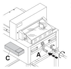
Tighten the backgauge crank ( $\bf A$ ). Parts and tools are in the tool set ( $\bf C$ ).
