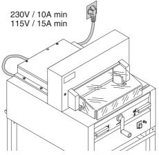
Connect the power cord to a single phase socket.
