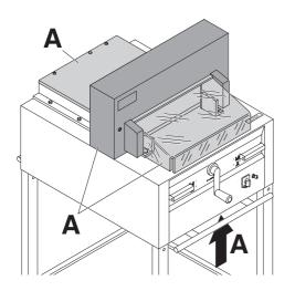
All components which could endanger the operator are covered by a guard!
