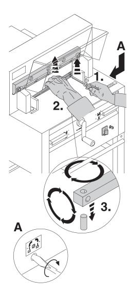
Take out the cutting stick with a small screwdriver. If needed the cutting stick can be turned or exchanged.
