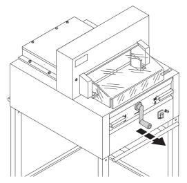
Pull out the handle to avoid the measurement being wrongly adjusted.
