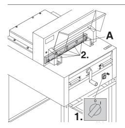
Tighten the blade screws  $(\mathbf{A})$  on the right hand side.
