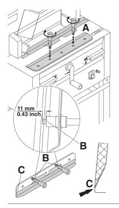
Take the exchange blade carefully out of the blade box and screw it to the blade changing tool (A).
