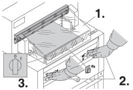
Close the safety guard (1.) Lower the blade by pressing both cutting buttons (2.). Keep one button pressed and turn off the main switch (3.).
