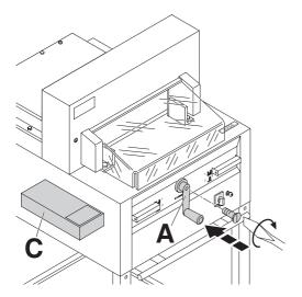
Tighten the backgauge crank (A). Parts and tools are in the tool set ( $\bf C$ ).
