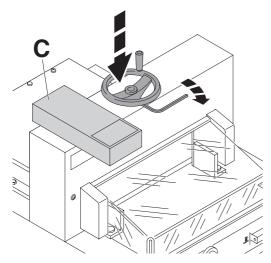
**Only 4815**Attach the enclosed hand-wheel for clamping. Parts ans tools are in the tool set (**C**).
