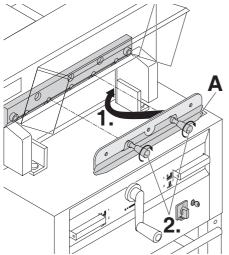
Place the blade to be exchanged with the blade changing tool (A) mounted (1.), into the blade carrier and push it up to the top and screw it into place with the grips (2.).
