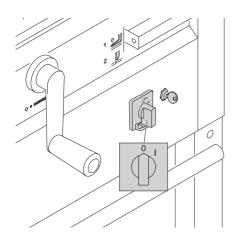
Replacement of blade and cutting stick may be performed only when the main switch is switched off!
