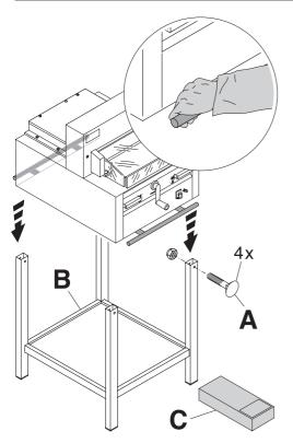
4 strong people are required to lift the machine from the pallet and place it on the stand. Secure with 4 screws (A). Put the shelf (B) on the stand. (Parts and tools are in the tool set (C).
