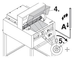
Open the safety guard (4.). With the special wrench (B) the 3 eccentrics should be screwed down (5.) until the paper is cut along the entire length of the blade (The blade must remain parallel, not too deep into cutting stick).
