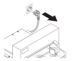
Disconnect from the mains before starting any service work or before removing the panels!
