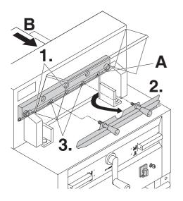
Lightly tighten 2 of the 5 blade screws (1.). Remove the blade changing tool (2.). Lightly tighten the remaining blade screws (3.).
