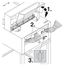
Close the safety guard (1.). Lower the blade by pressing both cutting actuators (2.). Keep one actuator pressed and turn off the main switch (3.).
