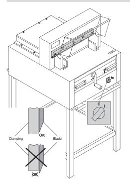
Remove the special wrench and turn on the main switch until the blade returns to the home position.
