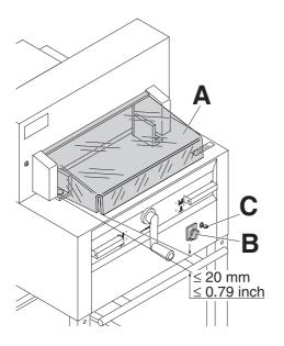
Before working with the machine and after every blade replacement the automatic cut-off function of safety guard (A),(correct if distance between cover and table is < 20 mm) main switch (B) and control panel (C) must be checked.
