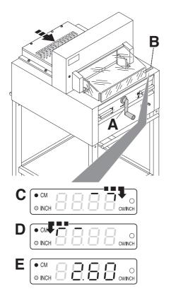
The measurement is set with the backgauge crank.(A) The symbol – rotary direction – ¬¬ moves to the right on the display (B) (see picture C). The rotary direction of the backgauge crank (A) is indicated on the right. Keep turning the backgauge crank to the right until a measurement appears (see picture E). The reference position is reached. The cutting size can now be set with the handle (A).
