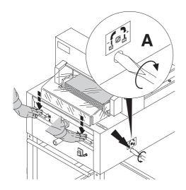
Paper cutting test. If the last sheet or several sheets are not completely cut, gradually turn the knob for blade depth adjustment (A) ¼ turn to the right until the paper is cut along the entire length. Do not set too low as blade will become blunt sooner.
