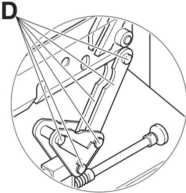
Grease the backgauge (A) control weekly with a grease gun. Advance the backgauge as far as possible to the front. (Use non-resinous oil or grease). Grease the remaining parts twice a year (see picture). The main switch must be on "0" (B). Remove lower panel (C).
