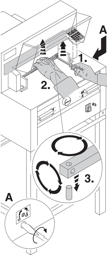
Take out the cutting stick with a small screwdriver. If needed the cutting stick can be turned or exchanged. (The cutting stick can be used 8 times).
