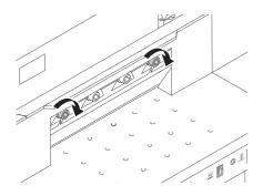
Slightly screw in outer screws.
