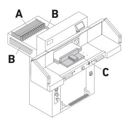
The stack of paper can be placed against the back gauge ( $\mathbf{A}$ ) and the left or right side stop ( $\mathbf{B}$ ). Use the supplied paper knock-up block ( $\mathbf{C}$ ) to move the stack of paper.
