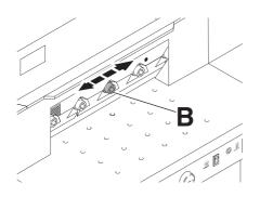
Push the blade and screw ( $\mathbf{B}$ ) as far as possible to the left or right and then centralize them.  $\rightarrow$  The blade must rest on the cutting stick.
