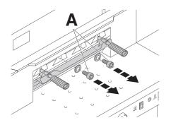
Remove remaining two screws (A).
