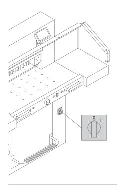
When not in use for a longer period switch off. (Main switch to " $\mathbf{0}$ ").
