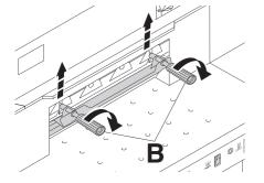
... and tighten with screws (B) in upper position.
