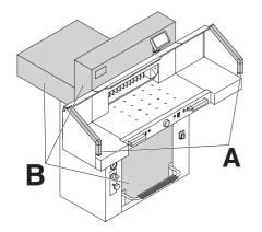
All components which could endanger the operator are covered by a guard (**B**)!
