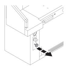
Pull out blade locking key  $\rightarrow$  blade moves to the top.
