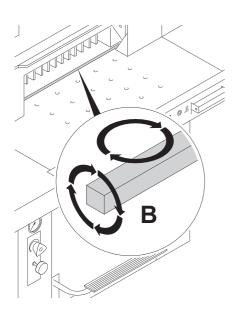
... or turn / replace the cutting stick (B). (See page 29 "Blade and cutting stick replacement").
