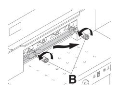
Simultaneously slightly loosen both screws (B) and remove blade with blade changing tool. Weight of blade approx. 5 kg.
