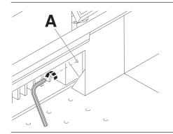
Paper cutting test. If the last sheet or several sheets are not completely cut, gradually turn the knob for blade depth adjustment (A) 1/6 turn to the left until the paper is cut along the entire length. Do not set too low as blade will soon become blunt.
