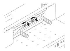
Screw in middle screws and tighten.
