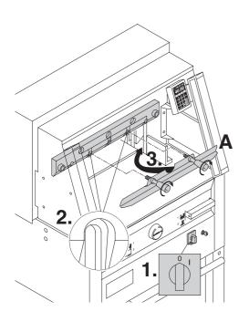
Position the main switch to "0" (1.) Remove the 2 blade screws on the elongated holes (2.). Then put the blade changing tool (A) into place and fasten it to the blade (3.).
