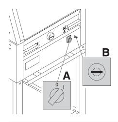
Main switch to position "I"? (A) Control system activated? (B) (Turn key to the right) Release a cut see page 21.
