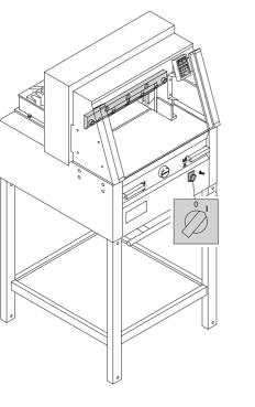
Remove the special wrench and turn on the main switch until the blade returns to the home position.
