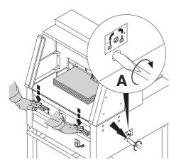
Paper cutting test. If the last sheet or several sheets are not completely cut, gradually turn the knob for blade depth adjustment (**A**) ¼ turn to the right until the paper is cut along the entire length. Do not set too low as blade will become blunt sooner.
