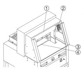
After 30 minutes the machine (1) (2) (3) (4)switches to energy-saving mode. The machine is reactivated by touching the keypad area (2).
