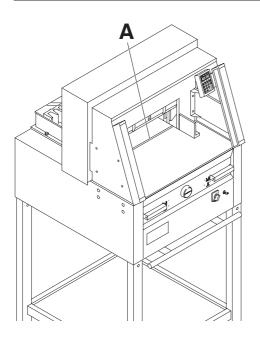
Cut is indicated by means of an optical light beam (**A**).
