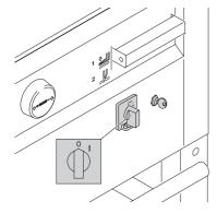
When not in use for a longer period switch off. (Main switch to "0").
