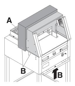
Operating the machine without safety device is forbidden! (Rear screwed safety guard (**A**) and panel (**B**)).
