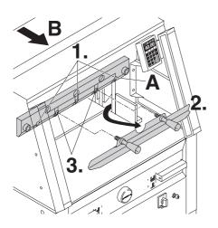
Lightly tighten 3 (4860 has 2) of the 5 blade screws (1.).
