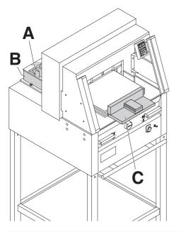
The stack of paper can be placed against the back gauge (**A**) and the left or right side stop (**B**). Use the supplied paper knock-up block (**C**) to move the stack of paper.
