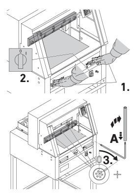
Lower the blade by pressing both cutting buttons (1.). Keep one button pressed and turn off the main switch (2.).
