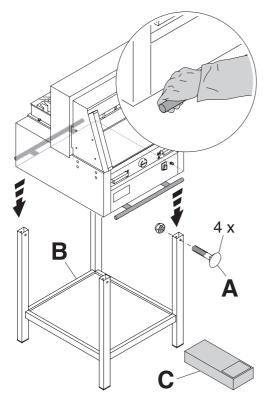
4 strong people are required to lift the machine from the pallet and place it on the stand. Secure with 4 screws ( $\mathbf{A}$ ). Put the shelf ( $\mathbf{B}$ ) on the stand. (Parts and tools are in the tool set) ( $\mathbf{C}$ ).
