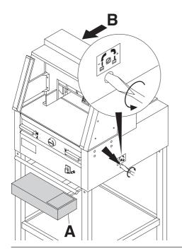
Turn the blade depth adjustment screw to the left until it stops. (Screwdriver found in tool set (A)) or tool holder (B).
