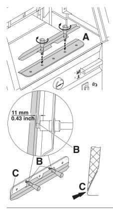
Take the exchange blade carefully out of the blade box and screw it to the blade changing tool (A).
