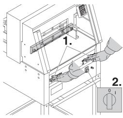
Lower the blade by pressing both cutting actuators (1.). Keep one actuator pressed and turn off the main switch (2.).
