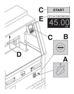
Position the main switch to "I" (A). Insert the key for the control system and move it to the right (B). The machine is now ready for use.
