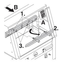
Lightly tighten 3 (4860 has 2) of the 5 blade screws (1.).
